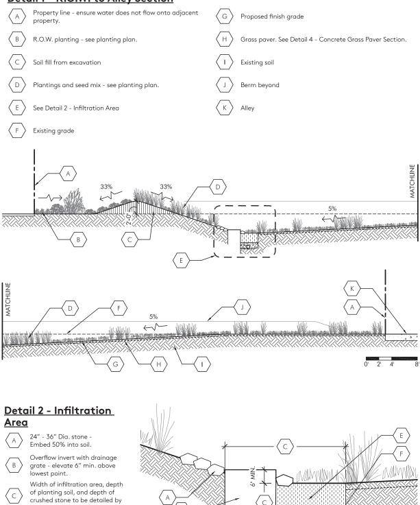
С engineer. В Perforated drainage pipe. Consult engineer for С specification and size. Rain garden planting soil D 3/4" dia. clear crushed stone, or 0' .5 1 2 as specified by engineer
